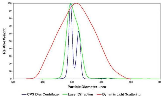
*Ultra High Resolution Capability - resolution comparison with Laser Diffraction and Dynamic Light Scattering*
